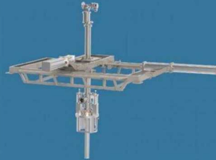
TH type electrically, hydraulically, pneumatically operated onspot railcar loading system.
